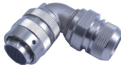
CKP08M14-19PT50 90° Plug with Emi Shield and Shrink Boot backshell
